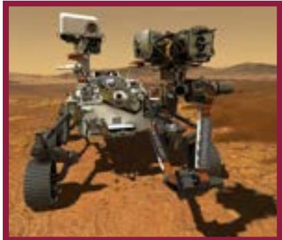
Ceramics experts in Stoke on Trent developed very accurately calibrated coloured tiles that are mounted on the rover. The 'Mastcam-Z' camera on the rover uses the tiles as a reference to ensure that the images that are sent back to Earth are showing the same colours that human eyes would see if we were there in person.
